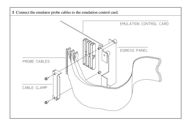
2 When inserting cable connectors into the sockets, press inward on the connector clips so that they hook into the sockets as shown. The order of connecting cables was given in step 1.
