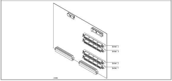
2 To ensure correct installation of optional memory modules on the deep analyzer card, there is a cutout at one end of the memory modules so they can only be installed the correct way.
